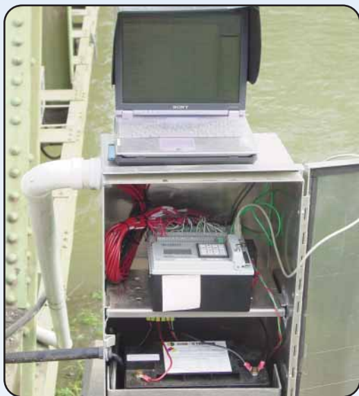
BDI-FMS mounted in semi-permanent cabinet. Other enclosure options available.
