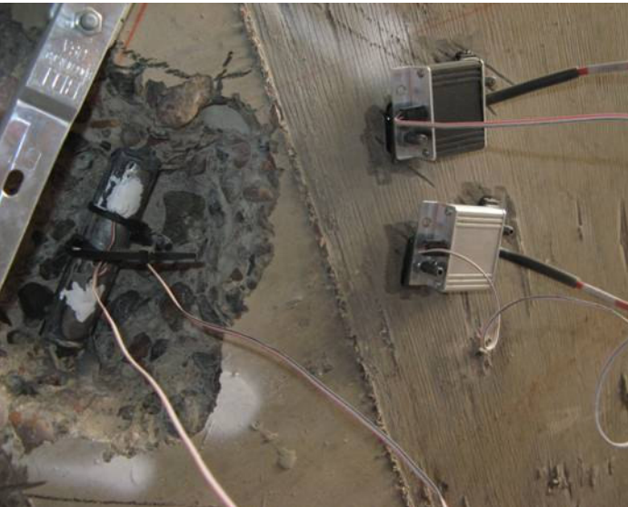
Quarter Arm Foil Gage on Reinforcing Steel
